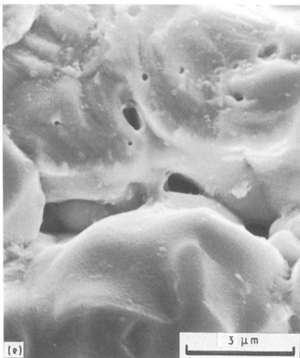
Figure 2 SEM micrographs of HIPed ZrN materials: (a) obtained by secondary electron emission (Cerac powder; 1600 °C, 190 MPa, 1 h), (b) fracture surface (Starck powder; 1600 °C, 195 MPa, 1 h), (c) fracture surface (porosity 8%, Cerac powder; 1600 °C, 120 MPa, 1 h), (d) fracture surface (Cerac powder; 1750 °C, 195 MPa, 1 h) and (e) bridging effect due to the viscosity of the oxynitride phase (porosity 6%, Cerac; 1550 °C, 1900 °C, 1 h).
